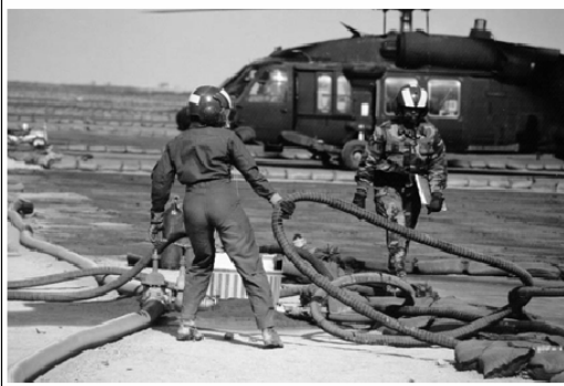
Fuel handling personnel moving fuel lines, 101st Airborne Division Rapid Refuel Point
