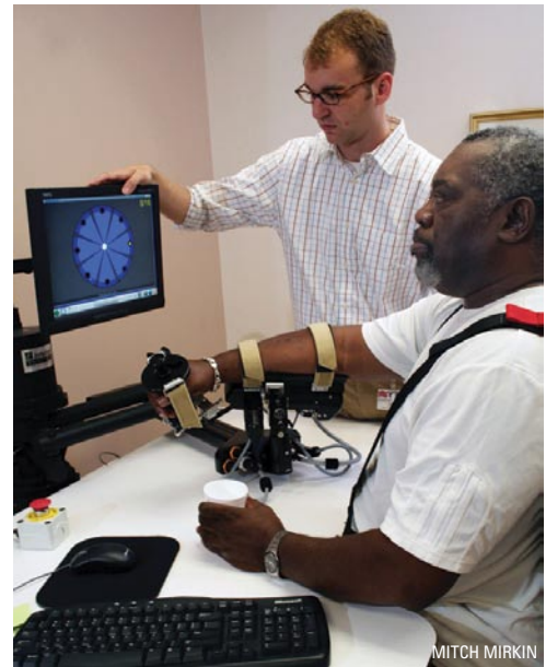
Allen Wright, a Navy veteran who suffered a stroke in 2000, exercises his affected arm with the use of a robot called the MIT-Manus, as exercise physiologist Tim DeHaan observes his progress. Wright is among more than 150 veterans taking part in a VA-funded clinical trial comparing robotic therapy with intensive non-robotic therapy for improving motor function in chronic stroke patients.
