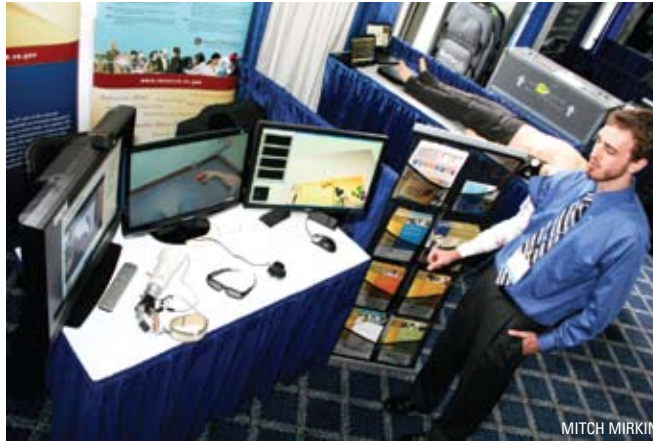
Joris Lambrecht, of the Cleveland FES Center, controls a virtual prosthetic arm on the screen through electrical signals from his shoulder muscles. The virtual system, based partly on video game technology, helps amputees learn to control a multi-joint prosthetic arm through impulses from their residual arm muscles.
