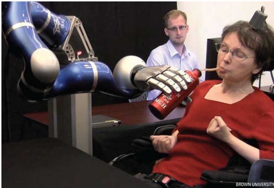
A 58-year-old woman, paralyzed by a stroke for almost 15 years, uses her thoughts to control a robotic arm, grasp a bottle of coffee, serve herself a drink, and return the bottle to the table.
